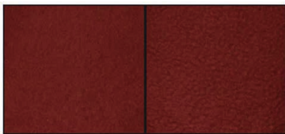
Figure C.2 — Example of matting appearance of napped fabric (back side): original (left) versus matting appearance(right)
