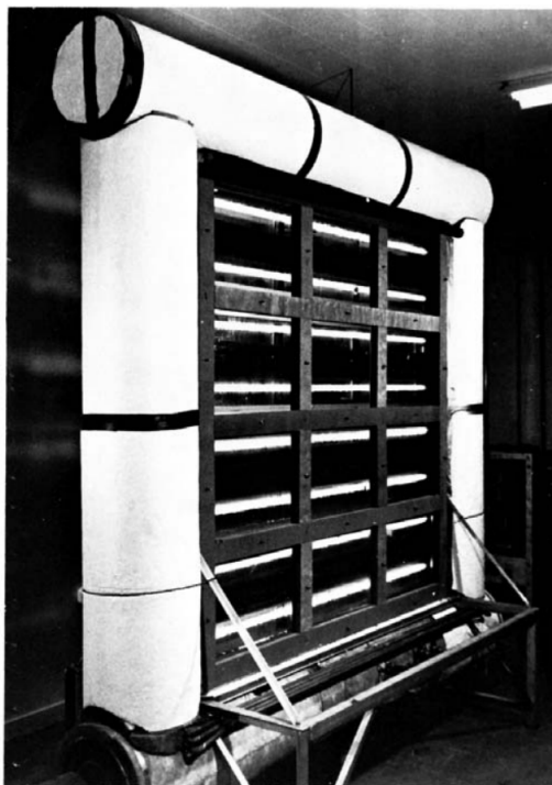
FIG. 1 Typical Accelerated Weather Cycle Test Apparatus
